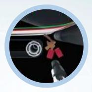
LOOP SENSOR CONTROL Controls media alignment throughout printing to help maintain high quality on heavy, coated, and banner stocks.
