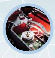
R-VCSEL LASER TECHNOLOGY Advanced 32-beam red VCSEL laser delivers 2,400 x 2,400 dpi, outputting detailed colour images with outstanding definition at high speeds.
